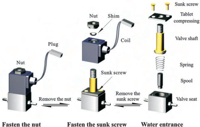
Picture 5 The assembly and disassembly of the solenoid valve
